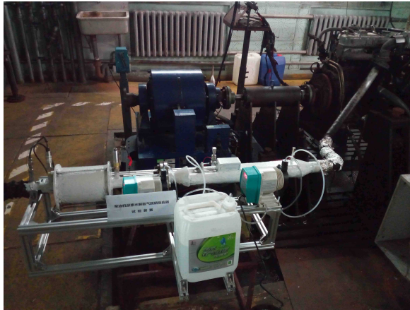
Fig. 5. Engine bench with urea hydrolysis SCR treatment
